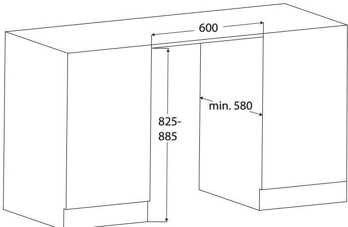
The kitchen cupboard must be aligned horizontally and vertically.
