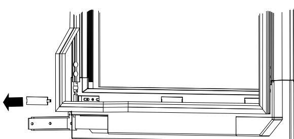
3. Remove the screws in Position 2 and move them to Position 3. Remove the screws in Position 1 and align the door,
