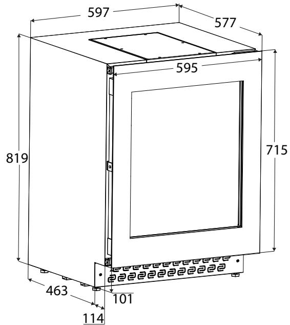
\*The adjustable feet can be used to increase the installation height to max. 879 mm.
