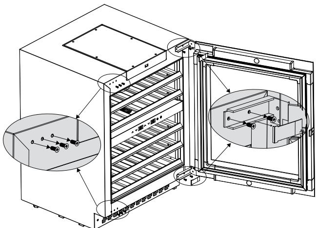
4. Remove the door and rotate it 180°.
