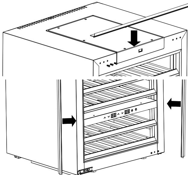
9. Slide the appliance until it is completely in the cabinet. Check all the gaps around the appliance. Use the spacers to position the appliance flush to the front of the cabinet. Loosen the screws (1), slide the spacers towards the side of the cabinet and then continue tightening the screws.
