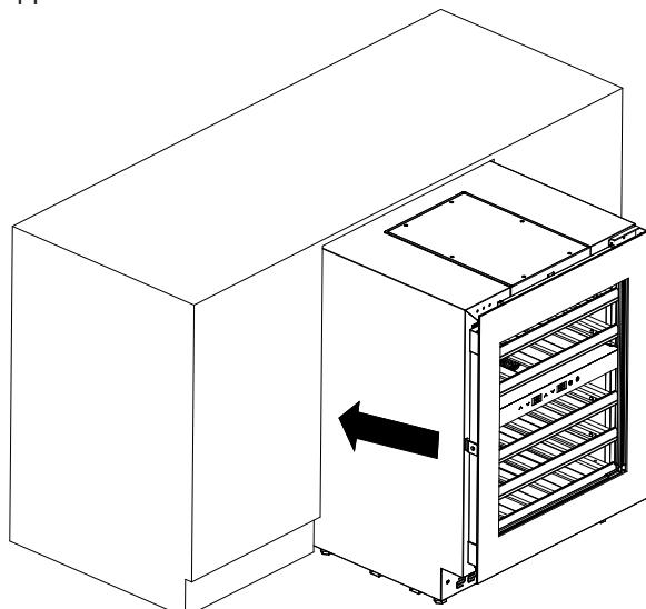
3. Unscrew the adjustable feet using the spanner provided until the appliance is flush with the top of the furniture body. If necessary, pull the appliance out of the recess.
