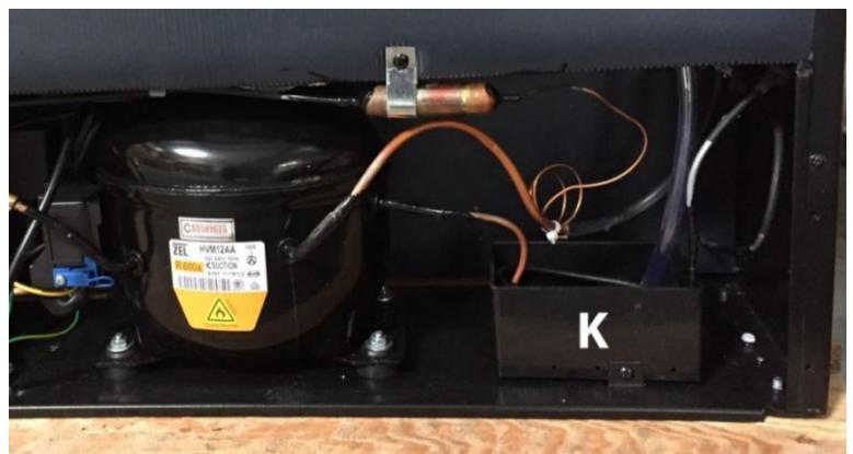
If necessary remove the condensed water with a sponge from the container for condensed water. The container is located on the back side of the device at the right bottom. Please remove the metal cover and then screw it back on.
