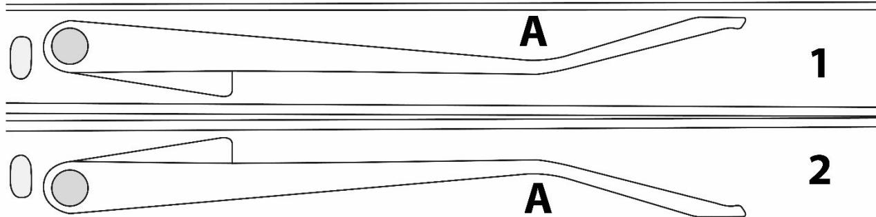
1 = below - release with pressure at point A upwards
