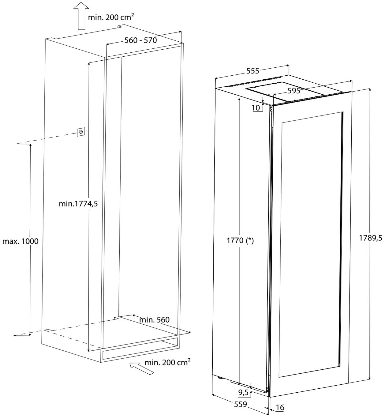
\*The installation height can be increased by the adjustable feet up to 1785 mm.
