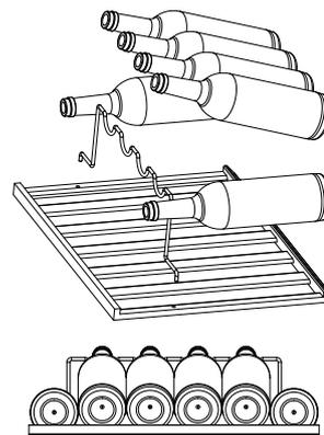
When it is time to display the bottle, you need to take out the upper shelf first, insert the metal bracket into the mounting hole of the shelf, and then lean the bottle against the bracket. Because both sides of the bottle will touch the upper guide rail, all can only be placed flat. The presentation rack is included in the scope of delivery.
